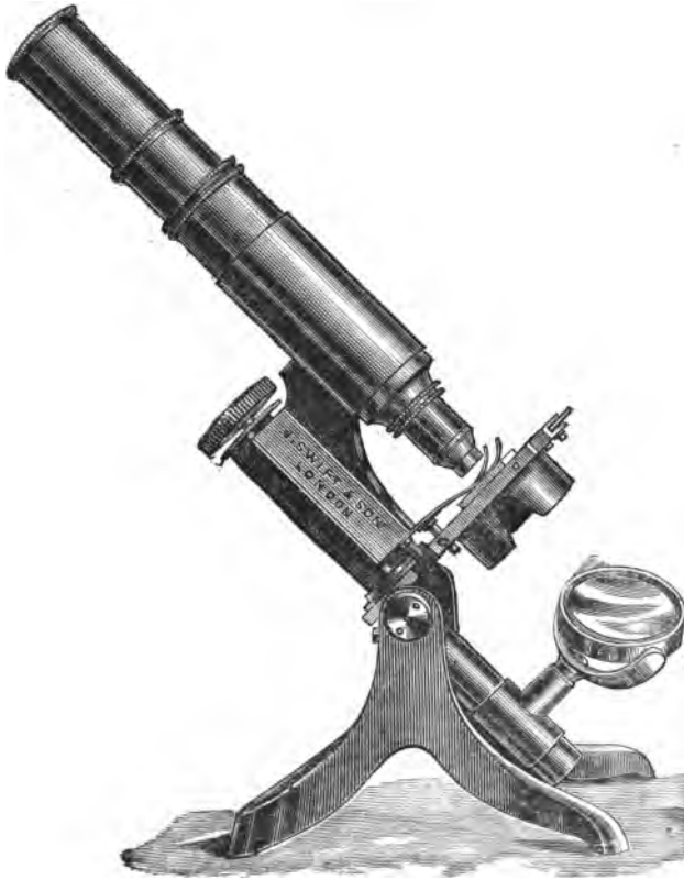
FIG. 15.—New College Microscope, by Swift & Sons—Tripod Stand.
